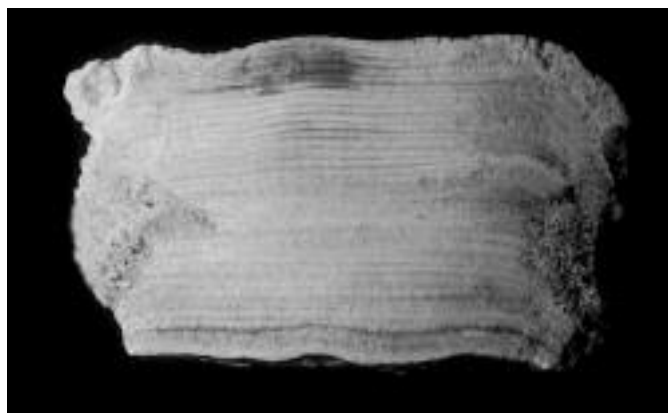
Figure 1: Cross section of a 30-years old stalagmite (5 cm high) of the Godarville tunnel (Belgium). It is annually laminated with an alternation of dark translucent compact and white porous layers.
